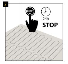
Before installation, turn off the underfloor heating for 24 hours.
