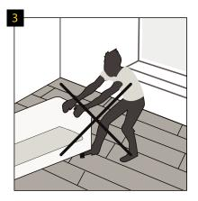
The movement of heavy objects along the floor is not allowed. They must be moved only after they are lifted.
