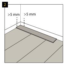
Leave 5 mm of perimeter space at the walls to allow the floor expansion. The maximum surface which can be laid without additional expansion joints is 200 m<sup>2</sup>. Above this surface, apply an additional expansion joint and enlarge all the expansion joints up to 10 mm. The maximum length of the floor surface in one direction, which can be laid without additional expansion joints is 20 m. Above this length, apply an additional expansion joint and enlarge all the expansion joints up to 10 mm.
