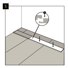
Then lower the panel in such a way as to fasten the lock on the short side, gently pressing the panel with fingers, starting from the corner and then towards yourself. The lock on the short side is provided with a special catch, which gets snapped if properly assembled. NOTICE! Do not use excessive force! If there are any difficulties with the lowering of the panel and closure of the lock, increase the clearance in the lock and lower the panel again.
