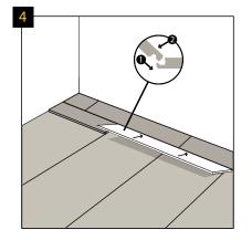
The Afirmax floor panels are provided with locks on the short and long side. First, connect the panel on the long side; for this purpose slide the long side of the panel into the groove of the previously installed row of panels. Move to the corner, leaving some clearance.
