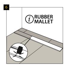
Use a rubberized hammer. Note! Each panel contains only 1 lock that can be pinned down. Other locks must be installed without driving in (see installation, Figure 4). Note! Try the lock very carefully before driving in (lack of precise fit of the lock and then driving the panel in will cause its damage, which will result in rejecting a possible claim).
