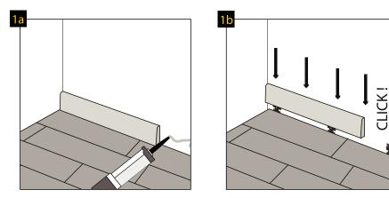
Expansion joints along the walls must be covered with a decorative strip, assembling it by means of glue or special clips. It is recommended to use the Arbiton strips dedicated to a given panel, which guarantee the excellent colour match and the coat resistant to scratching.
